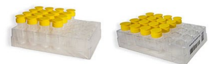
Fig. 2: AutoLys 24 well rack in SBS format for centrifugation of the Hamilton AutoLys M 1.0 tubes with the inner tube in lift and lock position (left) or for mechanical disruption of the MAP bacteria in the Hamilton AutoLys M 1.0 tubes in parking position (right).
