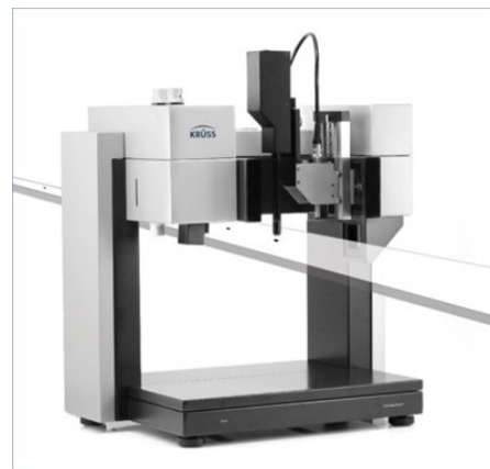
Fig. 1: Schematic setup of a series contact angle measurement on a moving sample.
