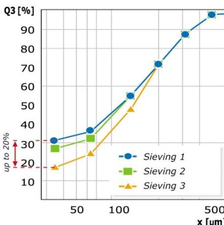
Reproducible sieving results due to digital setting of the oscillation amplitude
