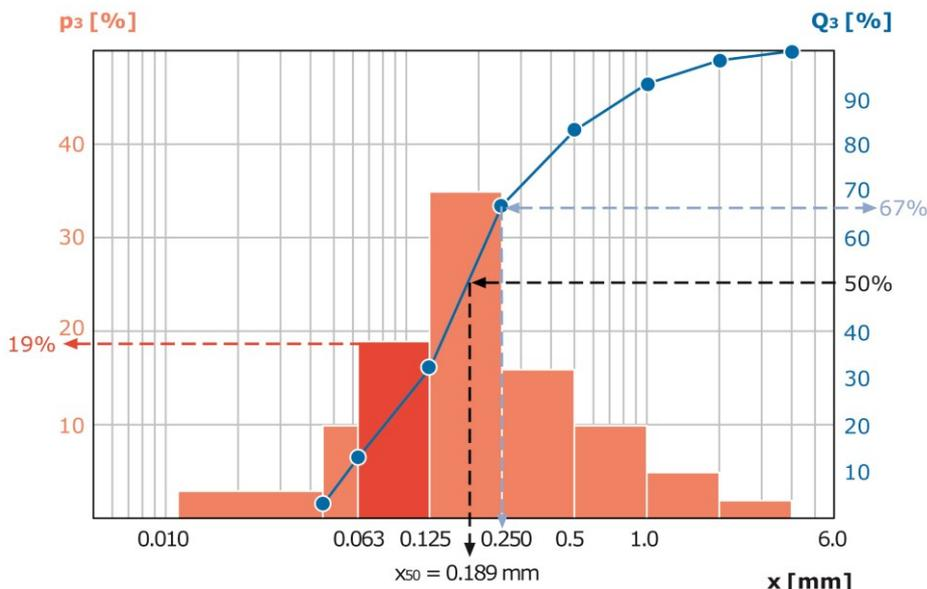
Fig. 7: Fractions  $p_3$  (left-hand y-axis) and cumulative frequency curve  $Q_3$  (right-hand y-axis)
