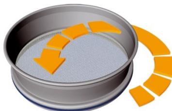
Fig. 4: In horizontal sieving the sample moves in horizontal circles.
