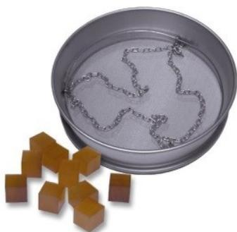
Fig.6 : Chain ring and rubber cubes are typical sieving aids
