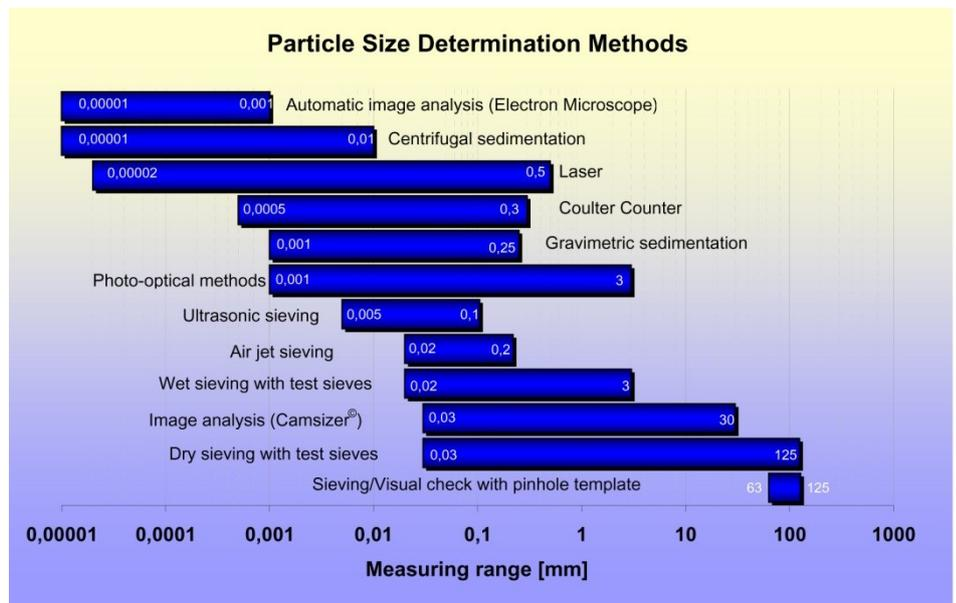
Fig. 1: Particle size determination methods
