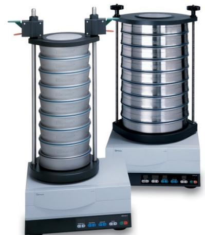
Fig.2: Retsch Sieve Shakers AS 200 and AS 300 control
