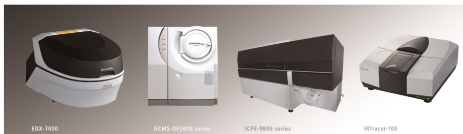
Fig. 2: Combined analytical techniques for analysis of different kinds of contaminants in plastics: XRF, ICP-OES, FT-IR, GC-MS
