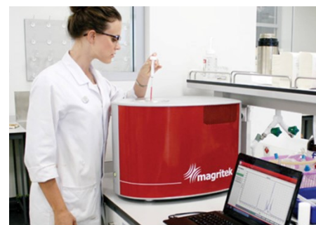
Fig. 1: Magritek Spinsolve benchtop NMR spectrometer.
