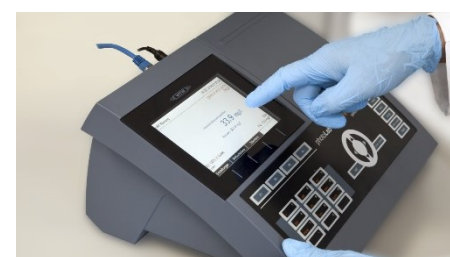
Fig.2: Results displayed for the parameters COD and nitrate after user calibration with the result and raw value
